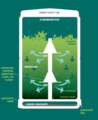
The Aerobin is a technological breakthrough. It uses a patented "lung" or aeration core within an insulated bin to promote aerobic and efficient break down of organic matter, which contributes to the reduction of greenhouse gas emissions.
